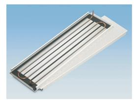
The contact cooling ceiling system KKS-3/LD is designed for combination with plane metal acoustic ceilings from various manufacturers to produce radiant cooling or heating ceilings or walls. The permanent large-surface contact between the cooling element and the ceiling tile is done with adhesive.
