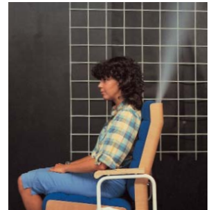
Air jet pattern of M-DJ
