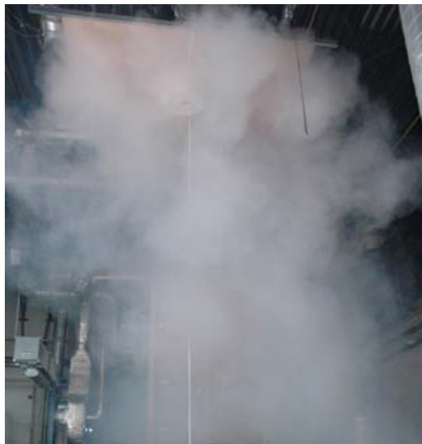
Fig. 6: Cooling mode with air outlet volume flow rate of 695 l/s [2 500 m³/h] and \Delta\vartheta_K = -5 K from 8.2 m height
