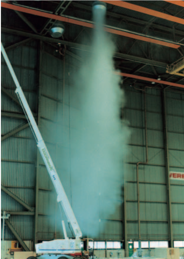
Fig. 8: Penetration depth of supply air jets made visible by smoke tracer
