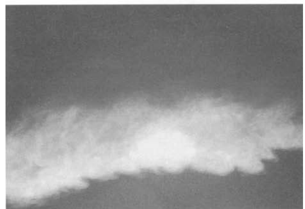
Fig. 6: Low-turbulence horizontal jet spread made visible by smoke tracer; the photographs show the air flow at various points in time after discharge
