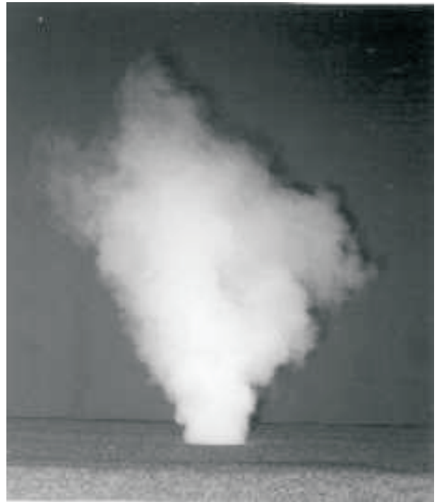
Figure 5: Jet pattern of floor twist outlet made visible with smoke tracer
