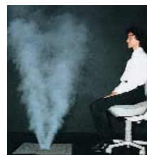
Jet pattern at various settings of the outlet
