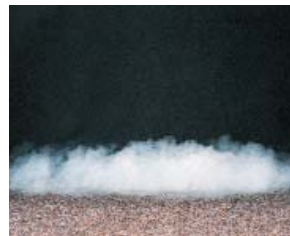
Air jet pattern "displacement flow"
