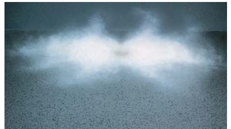
Air jet pattern of Q-B-DN 215
