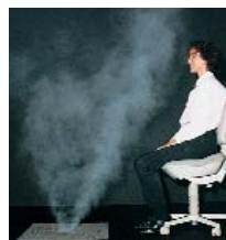
Jet pattern at various settings of the outlet
