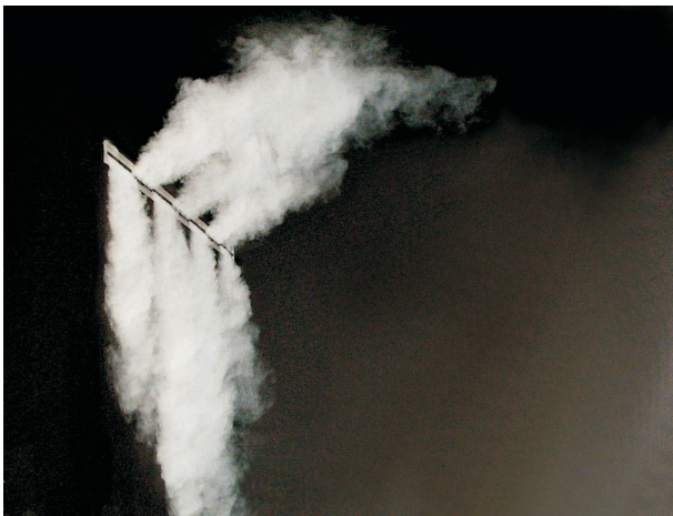
Fig. 5: Jet spread made visible by smoke tracer. Above: at an upward incline and downwards Right: horizontal
