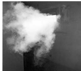
Jet pattern made visible with smoke tracer
