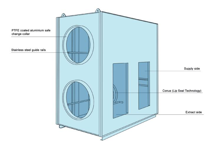
To guarantee the high efficiency of a HEPA filter element, the tightness of the filter seat is very important. The filter element is inserted onto stainless steel guide rails. ensuring alignment with the sealing spigot. The sealing spigot, also constructed from stainless steel is designed specifically to accommodate the inner seal ring on the circular filter element, which is locked into position during operation.
