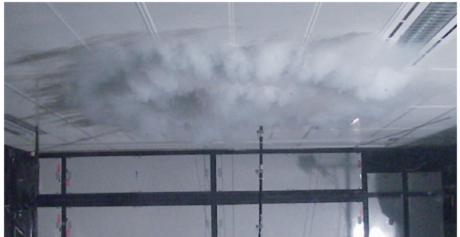
Air flow pattern made visible by smoke tracer
