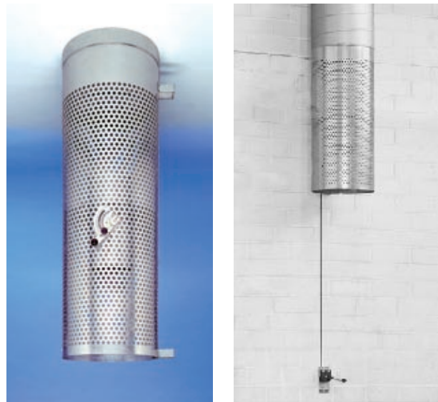
Fig. 2: Circular displacement outlet with adjustable damper left: adjustment with control lever right: adjustment with Bowden cable
