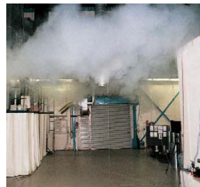
Air jet pattern of VA-ZD Cooling mode
