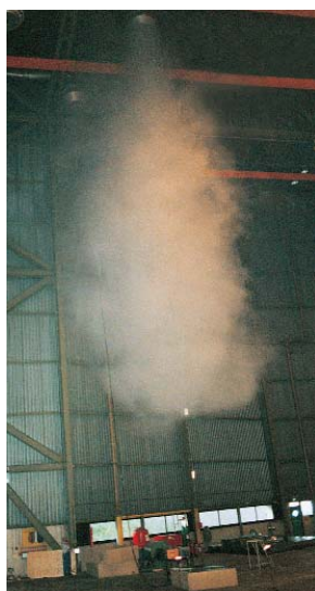
Air jet pattern of VA-K Cooling mode
