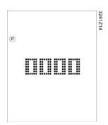
2. Press **Plus** or **Minus** to input password, press **Mode** to confirm it. If the password is correct, HMI-SG will show a new view for user to select group name.
