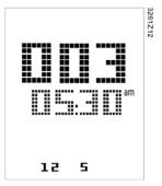
7. In scheduler setting, pressing PROG button will go back to the previous page. User can press this button to exit the setting step by step. HMI-SG will also exit time scheduler setting automatically if no operation was performed for 1 minute, and all changes made after pressing OK button will not be saved.
