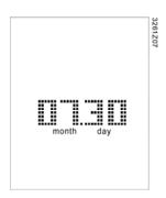
6. After the month and day is confirmed, HMI-SG will return to the view of time. Press button **PROG** or there is no any operation for 1 minute, it will exit the setting.
