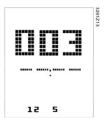
6. Press button **Plus** and **Minus** to set up time point and select an operation, and press **OK** to confirm the input. In any parts of time area, press **OK** when the cursor is located on "--" without a number is selected, the switch will be deleted, and HMI-SG will go back to viewing switch.
