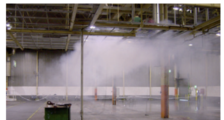
3 Low-turbulence displacement ventilation at a height of 3 m
