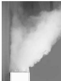
Fig. 2: Air upflow along the facade and air flow into the room, made visible by a sketch and smoke tracer
