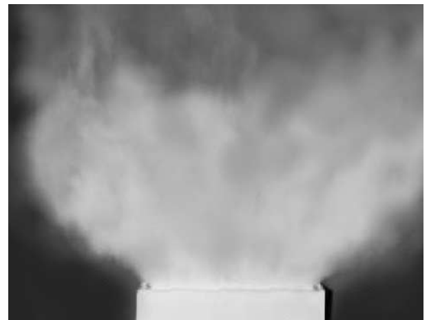
Fig. 3: View towards the facade, air flow made visible by a sketch and smoke tracer
